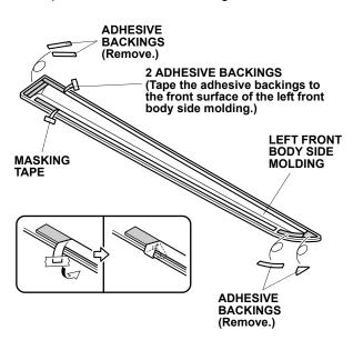
Align the left front body side molding with the template and attach it to the left front door as shown. NOTE: If the vehicle is equipped with door edge film, attach the left front body side molding at the indicated position.
