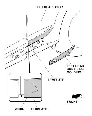
11. While applying light pressure against the left rear body side molding, carefully remove the taped adhesive backings.
