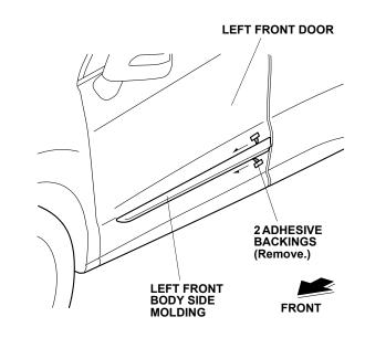
8. Using a rubber roller, apply pressure against the left front body side molding and roll from one end to the other.
