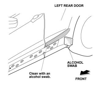
5. Peel back the adhesive backing from two adhesive strips, and tape the ends to the front surface of the body side molding with masking tapes. Remove the small pieces of adhesive backings.
